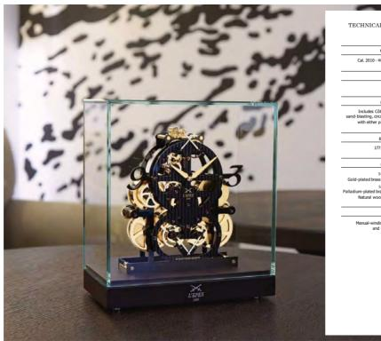
TECHNICAL SPECIFICATIONS MOVEMENT Cal. 2010 - 40 Days- 5 Barrels in serie JEWELS 46 FINISHINGS Includes Côtes de Genève, polishing, sand-blasting, circular and vertical satinfinishing, with either palladium or gold coating DIMENSIONS 177x 207 x 100mm MATERIALS 50 6595/001 Gold-plated brass movement, black main plates 50.6595/201: Palladium-plated brass movement, black main plates Natural wood base and Mineral glass WINDING Manual-winding: Design key to set time and wind the Barrels
